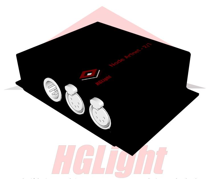
DmxNode - 2/1 has 2 outputs and 1 input DMX ports. It supports ArtNet and sACN protocols and can be configured with a web interface. It has many options, such as converting input to output, or using input and outputs simultaneously.
